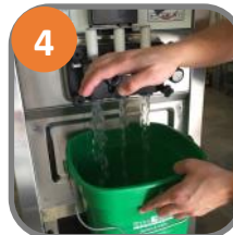
4 Drain Sanitizer Solution
