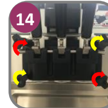
14 Install Dispensing Door Nuts (Diagonally)
