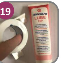
19 Lubricate & Install Hopper Agitators
