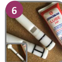
6 Install & Lubricate Draw Valves & Prime Seals
