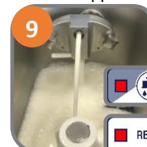
9 Press WASH to Prime Air Pump, Make Sure Product Pumps Out Strong, then Press RESET
