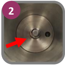
2 Install Drive Shaft into Cylinder, Rotate to Lock in Place
