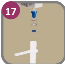
17 Install Suction Tube with Spring and Plug
