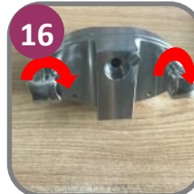
16 Install Pump Cover & Hand Nuts
