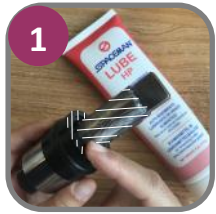
1 Install Drive Shaft Seal, Lubricate Drive Shaft & End of Seal (Shaded Area)
