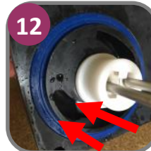
12 Install Door Gaskets and Front Bearings
