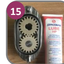
15 Install Gears & Seal Lubricate Seal Lightly
