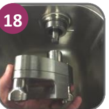
18 Install Air Pump Assembly (DO NOT INSTALL FEED TUBE)
