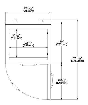
**Doors** Capacity Cu.Ft. 2 **Shelves** Refrigerant R-290 **Temperature** -10°F ~ 5°F Range Sliding Easy **Condensing Unit** Maintenance 9.8 ft long (3m) flexible three Connection wire cord with modeled plug HP 1/4 HP Voltage 115V/60Hz 3.2 **Amps NEMA** Config. NEMA 5-15
