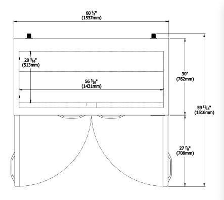
2 **Doors** Capacity 16.7 Cu.Ft. **Shelves** 4 Refrigerant R-290 **Temperature** -5°F ~ 10°F Range Easy Sliding Condensing Unit Maintenance 9.8 ft long (3m) flexible three Connection wire cord with modeled plug HP 1/2 HP Voltage 115V/60Hz 6.2 **Amps NEMA** Config. NEMA 5-15
