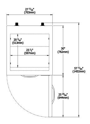
**Doors** Capacity Cu.Ft. **Shelves** 2 Refrigerant R-290 **Temperature** 33°F ~ 39°F Range Easy Sliding Condensing Unit Maintenance 9.8 ft long (3m) flexible three Connection wire cord with modeled plug HP 1/4 HP Voltage 115V/60Hz 3.6 **Amps NEMA Config.** NEMA 5-15
